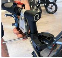
2 Snap the holder onto the upper part of the hand grip tube.
